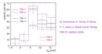
Time resolution of the detector crucial for separating ν<sub>e</sub> burst from the accretion phase signal
