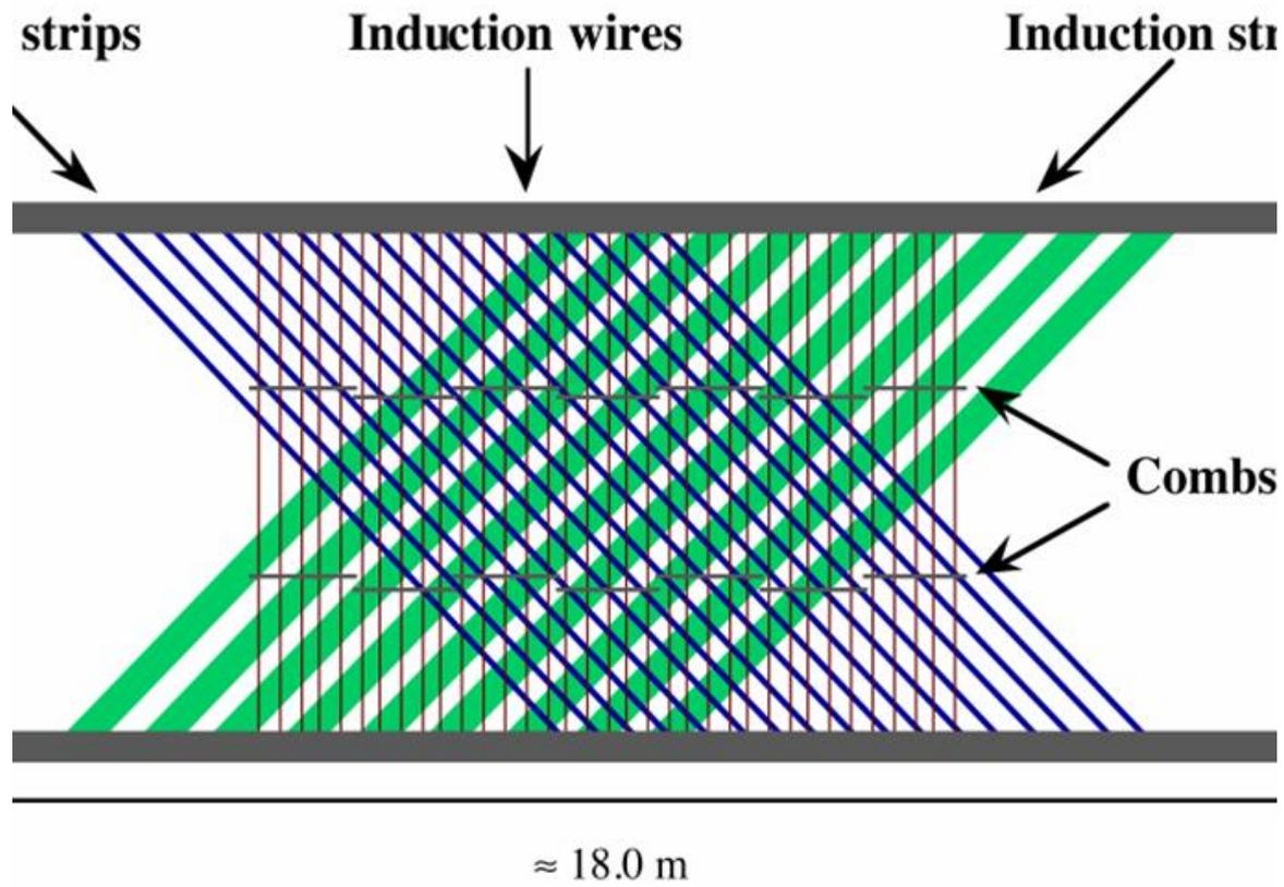
**Schematic layout of the “multi-layer + wires” read-out chamber**
