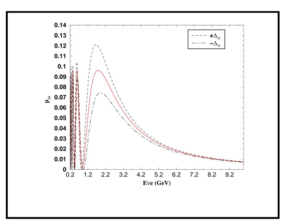
For  $\Delta_{31}$  positive this probability is higher and for  $\Delta_{31}$  negative this probability is lower than the vacuum expectation. Changing the sign of  $\Delta_{31}$  is leading to a change of about 25% in the oscillation probability.
