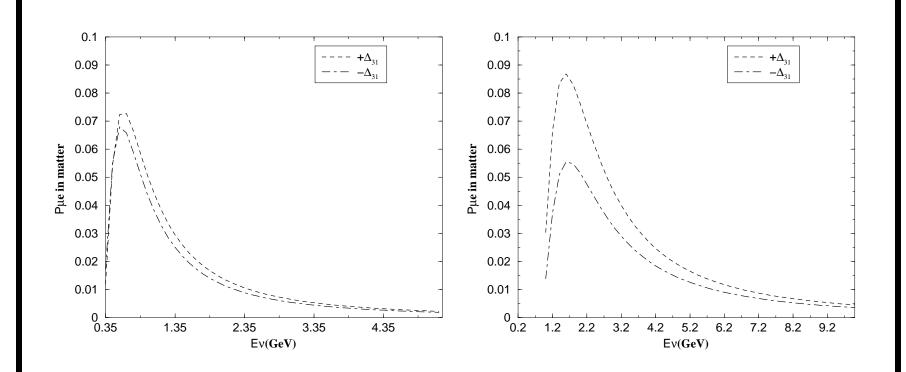
The figure on the left is for T2K and figure on the right is for No $\nu$ a.  $\Delta_{31}$  positive curve has  $\delta=30^\circ$  and  $\Delta_{31}$  negative curve has  $\delta=75^\circ$ . In both cases  $|\Delta_{31}|=2.5\times 10^{-3}~{\rm eV}^2$  and  $\theta_{13}=10^\circ$ .
