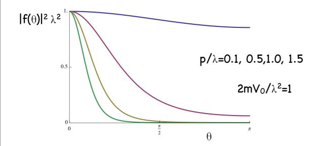
$$V(r) = \frac{V_0 e^{-\lambda r}}{\lambda r} \qquad f(\theta) = -\frac{2mV_0}{\lambda} \frac{1}{q^2 + \lambda^2}$$
