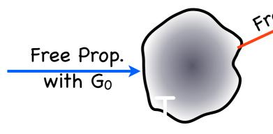
$$T = V[1 - G_0V]^{-1} = V + VG_0V + VG_0VG_0V + \dots = V + VG_0T$$
