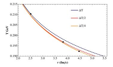
Temperature is plotted as a function of time. With peak value (a) of  $\zeta/s$  remains same while width ( $\Delta T$ ) varies. Solid line in the curve ends at the time of cavitation, while the dashed lines shows that how system would continue till  $T_c$  if cavitation is ignored. Figure shows that larger the  $\Delta T$  shorter the cavitation time.
