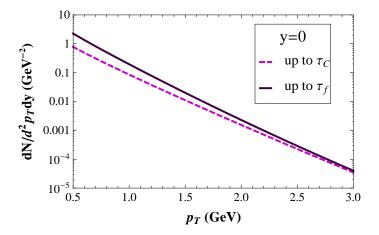
Photon spectrum obtained by considering the effect of cavitation (dashed line). For a comparison we plot the spectrum without incorporating the effect of cavitation (solid line). (At p=0.5 GeV overestimation of rate is 200% and at p=2 GeV it is 50%).
