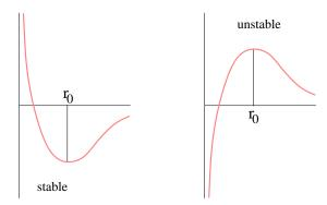
The stability of circular orbits depends on whether the orbit is at the local minimum or maximum of u. When it is at the minimum, small displacements give rise to simple harmonic oscillations around the stable orbit. This is an extension of the analysis of static stability to a non-inertial frame.
