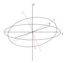
Take the xyz axes to be the inertial space frame. Orient the body frame XYZ along the principal axes. If the spin velocity around  $\hat{\mathbf{Z}}$ , is  $\dot{\gamma}$ . The line of nodes,  $\hat{\bf n}$ , is orthogonal to  $\hat{\bf z}$  and  $\hat{\bf Z}$ . The angular velocity along  $\hat{\bf n}$  is  $\dot{\beta}$ . The angle between  $\hat{\bf x}$  and  $\hat{\bf n}$  is  $\alpha$ .
