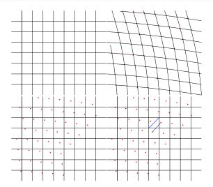
The instantaneous deformation of a body defines a tensor field  $u_{ij}$ .
