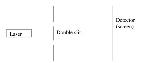
Use a laser which emits one photon at a time. Use the screen as a detector.
